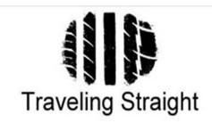
When traveling in a straight line, the shape of the contact patch is symmetrical to optimize traction and braking
